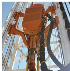
Cover Photo: A Horizon Drilling 600,000 lb hook load, Duvernay class, AC telescopic triple, walking pad rig. This rig has a depth capacity (TVD) of 6,000 metres (19,700'), a high-pressure circulating system rated for 52,000 kPa (7,500 psi), a multi-directional integrated walking system, and has been optimized for craneless rig up. The proprietary batwing top drive system is safer, lighter, and easier to maintain with an innovative extend feature that surpasses conventional designs.
